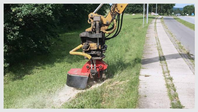
Increase your excavator's functionality by adding a hydraulic-powered stump cutter attachment, ideal for hard-to-reach areas such as slopes, riverbanks, or behind fences and stone walls. Our range accommodates excavators from 2-20 tonnes (15-160 hp).
