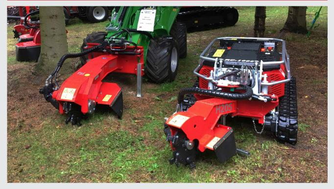
Maximise the versatility of your loader or tool carrier by adding a stump cutter as a tool, allowing stump removal in hard-to-reach areas. Two hydraulic cylinders and an adjustable flow valve ensure a stable sideways sweep controlled either directly from the tool carrier's controls or by an electronic switch box. The stump cutters come with an uncoated back plate, allowing for welding on a suitable attachment. A wide selection of tool attachments is optionally available upon request.
